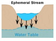
anticipate a recharge of 1,000 to 2,020 AF for the Project. To monitor the groundwater levels we will utilize monitoring wells along the streambed in several locations. Measurements will be taken weekly before, during, and after the water is released.
